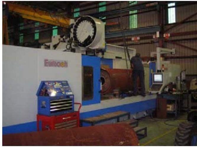
**Body Turning** – Done in house on either our largest Kinwa CNC lathe (pictured below) with 1980 diameter body capacity x 4000 long x 13Tonne body mass or on either of our 2 larger manual lathes which can produce quantities well in excess of whatever bodies are bored in a day.
