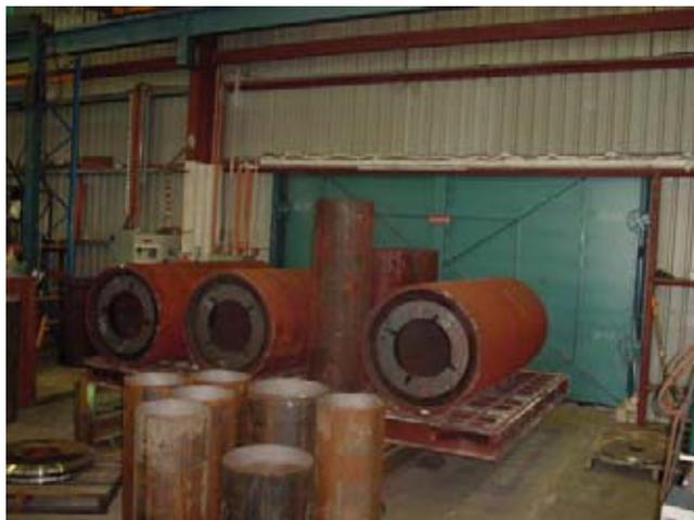
**Body Boring** – Done in house on our Union Horizontal borer or our Eumach FBE4000 or Eumach FBE3000 both of which have fully programmable heads to rough out bores and face each end under program before fine boring with special preset boring bars. Presently operating 2 shifts a day. We can bore at least 15 bodies a day.
