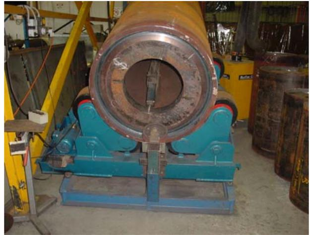
**End Disc to Shell external welding** – Done in house to our qualified and confidential weld procedure on either of our 2 automated Submerged Arc rigs which operate 2 shifts a day, presently doing up to 12 bodies a day. Maximum body mass is 20 Tonnes.
