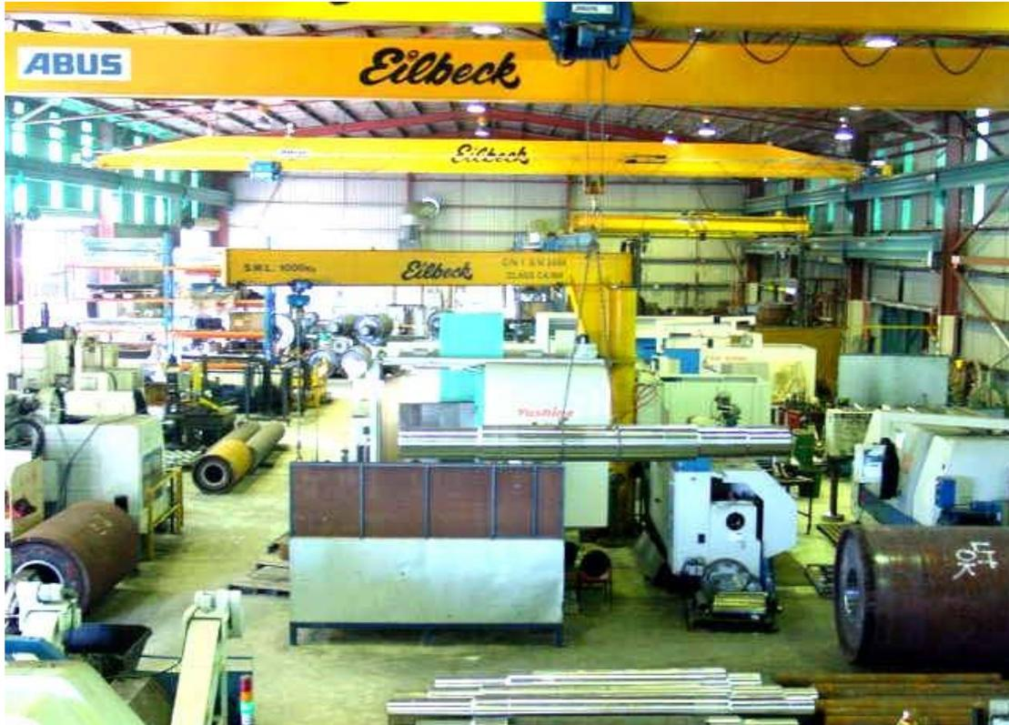
**End Disc Turning** – Done in house on either of 3 CNC lathes to 2500mm diam or our CNC 1250mm swing vertical lathe giving a combined capacity of more than 50 end discs a day.
