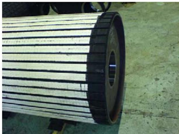
**Polyurethane Lagging** – Our subcontractor shot blasts the turned body OD and shell overhang to class 2.5, then fits a steel mould around the bodies and pours the hot cast degassed polyurethane into the mould before hot curing in their 3 ovens. After curing the poly which is moulded oversize is turned to the nominated diameter and lagging thickness and grooved if required.
