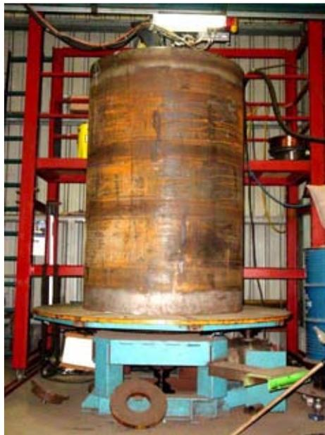
**Stress Relieving** - Done in house in our computerised gas fired stress relieving oven with internal dimensions of 4200 x 2600 x 2600.
