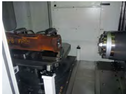
4 CNC Machining Centres with a Litz CNC Horizontal twin pallet (630x630) 4 axis machining centre shown on the left installed in 2009 and a Mitsubishi CNC Vertical Machining Centre shown on the right above with 1200 long x 800 vertical x 700 cross travels with a 500 diameter 4 th axis, 26Kw 6000RPM spindle and a 24-pot tool changer. 2 x Quantum CNC Vertical Machining Centres located at Ringwood with up to 1500 long x 900 vertical x 700 cross travels . All machines are fitted with a 4 th (rotary) axis for 4 side machining and are fitted with auto tool changers.
