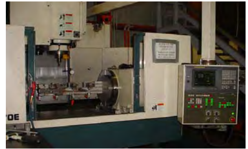
4 CNC Machining Centres with a Litz CNC Horizontal twin pallet (630x630) 4 axis machining centre shown on the left installed in 2009 and a Mitsubishi CNC Vertical Machining Centre shown on the right above with 1200 long x 800 vertical x 700 cross travels with a 500 diameter 4 th axis, 26Kw 6000RPM spindle and a 24-pot tool changer. 2 x Quantum CNC Vertical Machining Centres located at Ringwood with up to 1500 long x 900 vertical x 700 cross travels . All machines are fitted with a 4 th (rotary) axis for 4 side machining and are fitted with auto tool changers.
